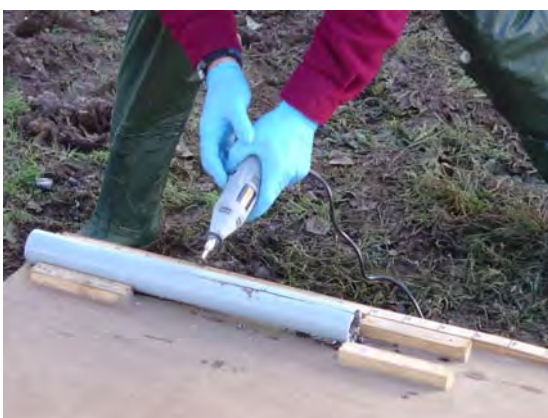
Figure 8.7 Sawing of the core in site (photo: Nick Riess).
