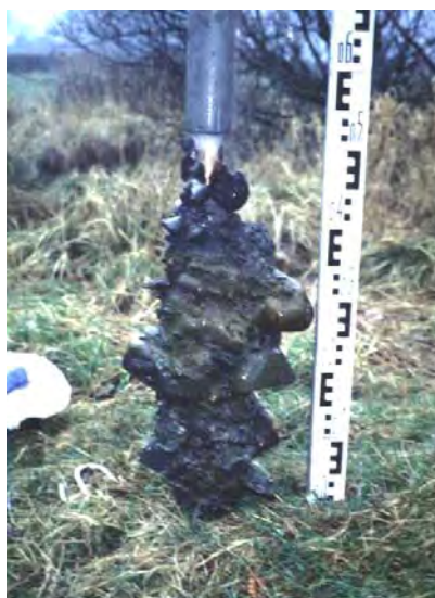
Figure 8.8 Ice coring; left: core being extracted; right: frozen core (photo: Andy Quin).
