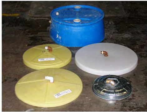
Figure 8.13 Four designs of low-profile seepage cylinder shown with a standard half-barrel seepage cylinder made from a plastic storage drum. From Rosenberry and LaBaugh (2008).
