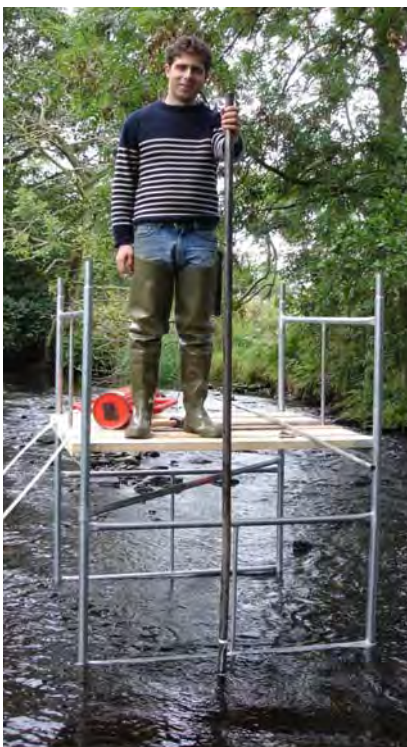
Figure 8.2 In-stream mini-piezometer installation on a scaffold tower. A drive-pipe fitted with a removable driving-point is hammered into the riverbed using a fence post-driver; at the required depth, the mini-piezometer is inserted in the drive-pipe, and the latter pull out by keeping the mini-piezometer in place (photo: Tristan Ibrahim).
