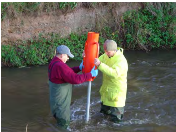
Figure 8.6 Hammering of PVC tube for coring of soft riverbed sediments (photo: Nick Riess).
