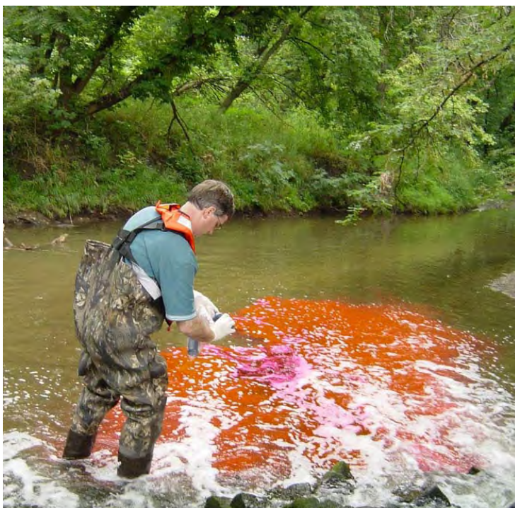
Figure 8.18 Adding Rhodamine WT dye to a stream. From http://toxics.usgs.gov/photo_gallery/instreams.html .
